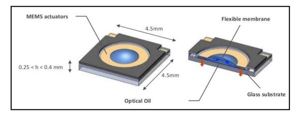
Wavelens indicates that its technology has numerous advantages over VCMs including compactness (4X more compactness), power consumption (1000X better) and reliability (no moving mechanical parts). In addition, Wavelens believes the cost can be dramatically less
