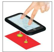
The ForceTouch Array is a MEMS sensor layer below the surface of the display, so it doesn't affect the optical clarity of the display. NextInput indicates that its technology is substantially less costly (in volume) and consumes about half the power of capacitive touch, and that it can work with a stylus, and in virtually any environment (high EMI location, underwater, etc.). The
