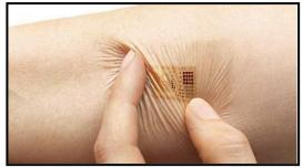
directly onto the skin without a person even noticing it while it is on. MC10 has developed technologies that allow extremely thin, flexible, conformal, transparent devices that can stretch, bend, and twist while on a person's skin. This has the potential to greatly accelerate the penetration of biosensors into several markets.
