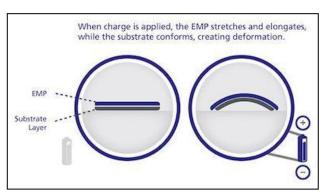
and can, therefore, act as both an actuator and a sensor. With digital control, the actuators can produce precise localized vibrations (the frequency of which can be varied), sounds, or deformation. It can also be used as a sensor to recognize touch/pressure.
