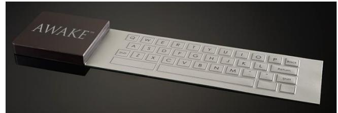
that incorporates haptics (can produce a variety of vibrations and sound effects when a key is touched). It is designed to replace conventional keyboards. According to the company, Novasentis has a variety of next-generation solutions in development that it believes have the potential to have a significant impact on the haptic market.
