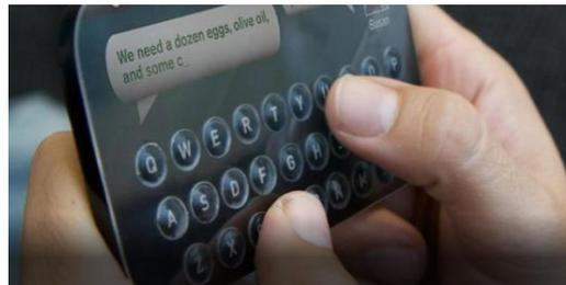
The underlying technology is based on microfluidics. Small transparent fluid channels are routed throughout the “Tactile Layer” and the fluid can expand the polymer layer above it to create physical buttons. A small controller chip is used to control the fluid channels and create or recede buttons. An API is provided to enable applications to control where and when buttons are created.
